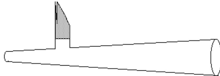
FIGURE 2: Absorption High. Cone tapered, minimum flare.
